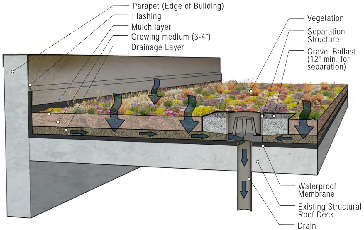
**FIGURE 4.7.3 - BASIC VEGETATED ROOF COMPONENTS**
