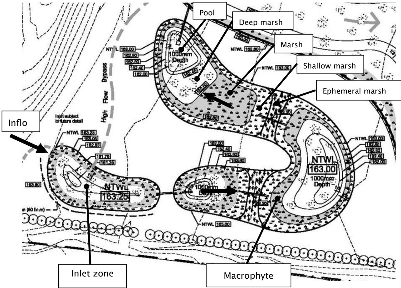
Figure 8.7. Example bathymetry of a constructed wetland system (GbLA, 2004)
