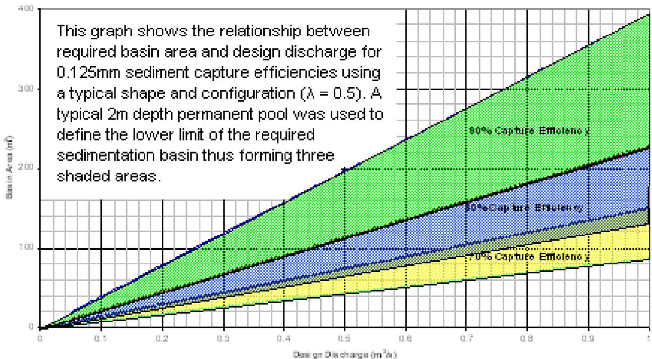
From above, the required sedimentation basin area to achieve target sediment ( $125 \mu\text{m}$ ) capture efficiency of 90% is  $50 \text{ m}^2$ . With a W to L ratio of 1:4, the notional dimensions of the basin are  $3.5 \text{ m} \times 14 \text{ m}$ . This figure correlates with the graph above.
