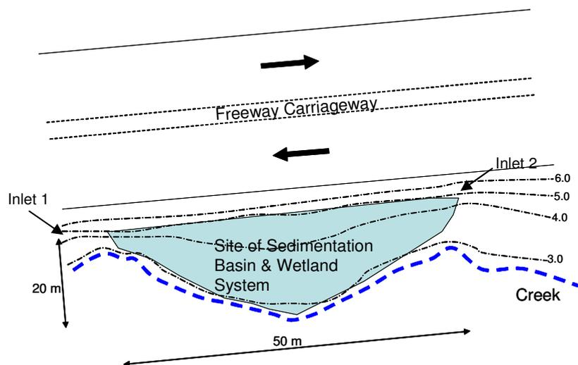
Figure 3.9 Layout of Proposed site for Sedimentation Basin
