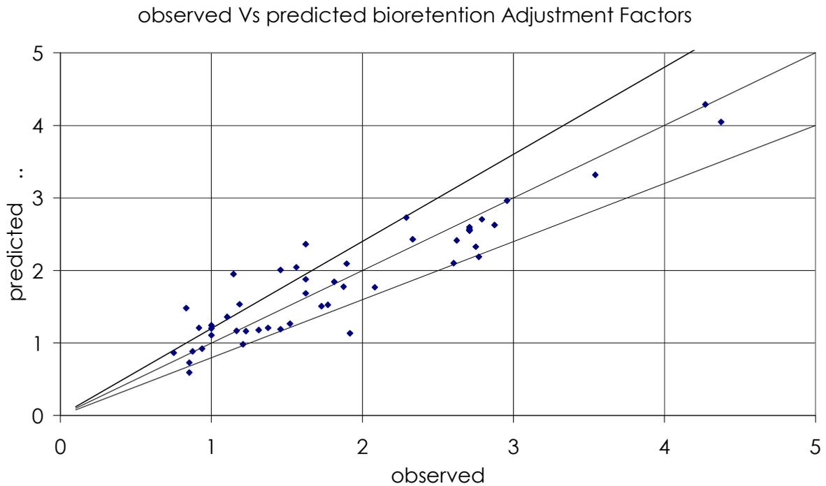
Figure A-12. Observed Vs predicted adjustment factors for bioretention systems
