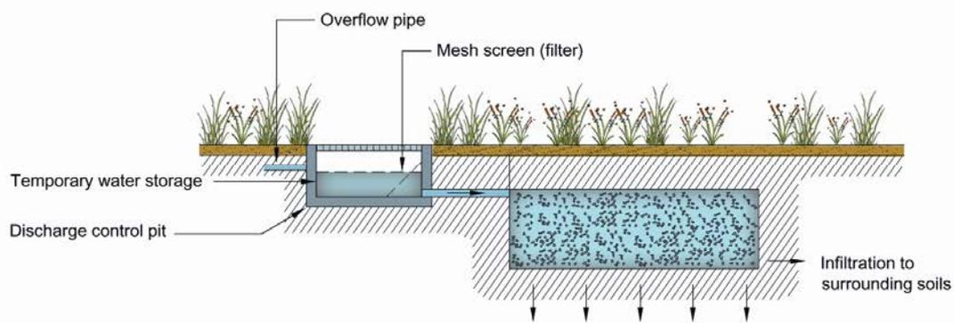
**Figure 10.1 Operation of a gravel filled 'soak-away' pit style infiltration system**
