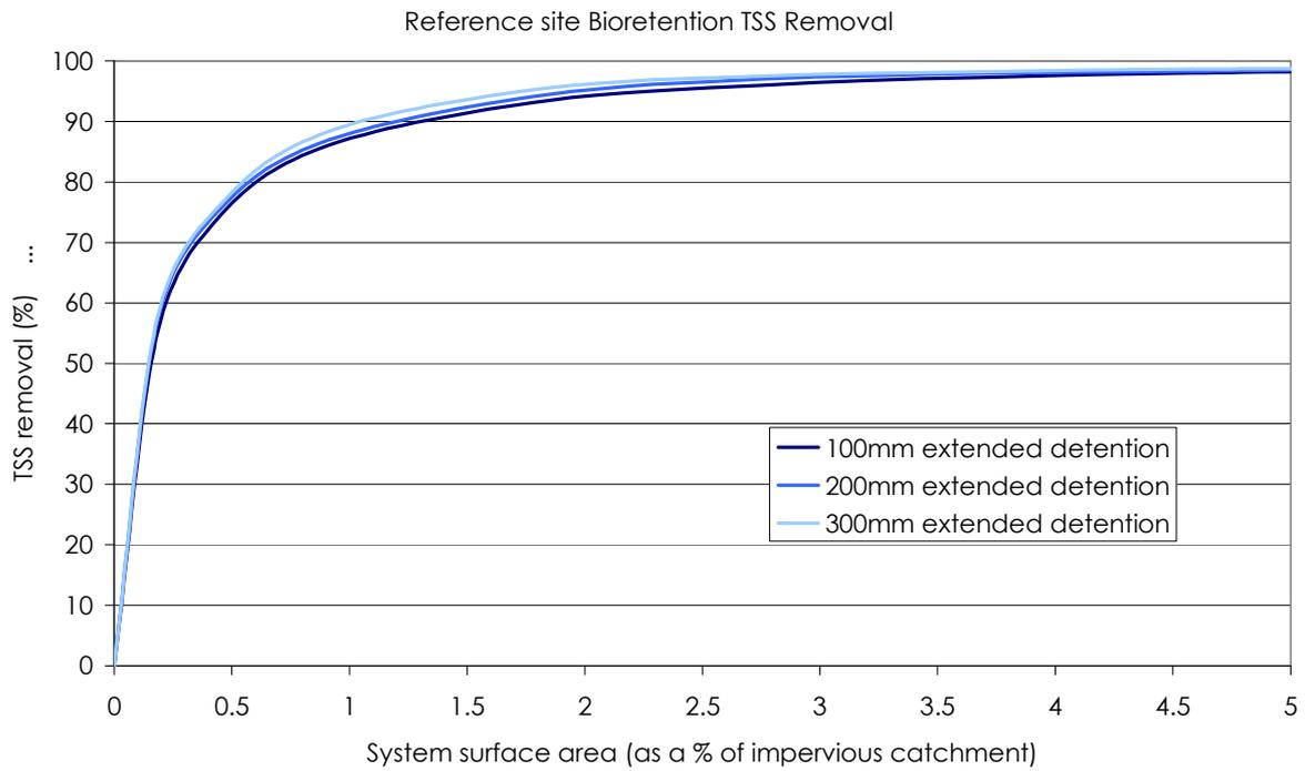
**Figure 5.3. TSS removal in bioretention systems with varying extended detention**
