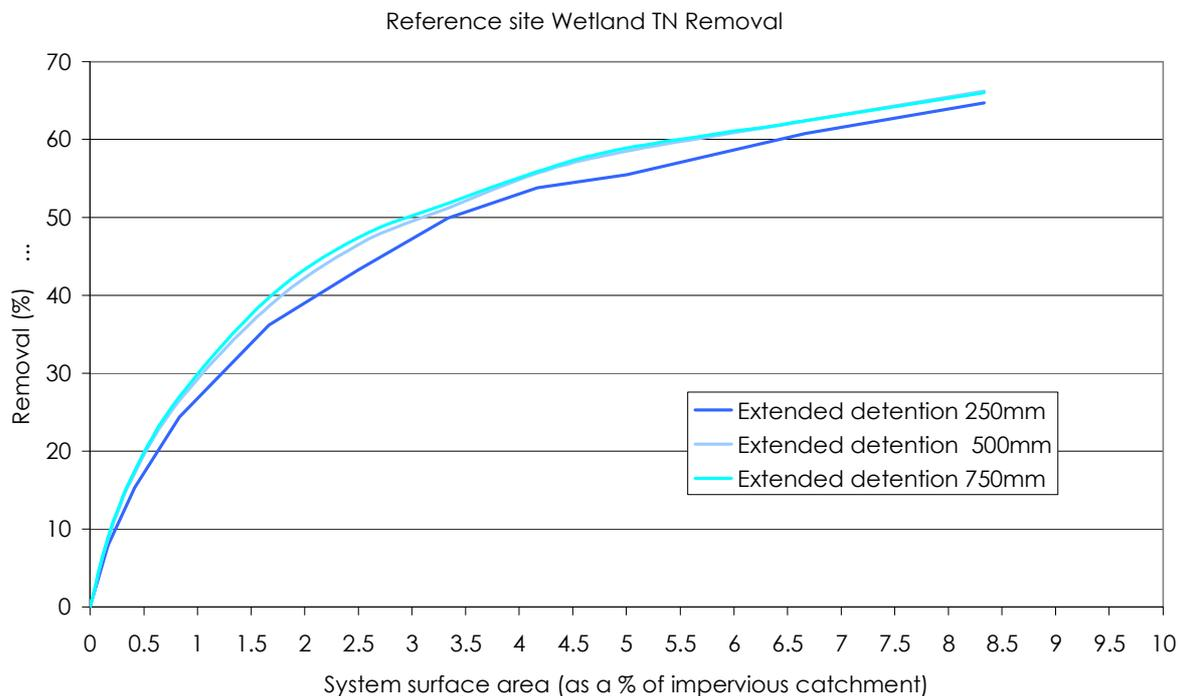
**Figure 8.4. TN removal in wetland systems with varying extended detention**
