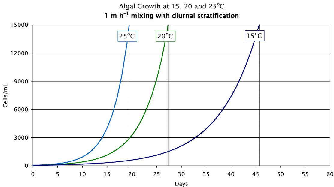
**Figure 9.4.** Growth curves illustrating modelled times for cyanobacterial populations to reach bloom proportions under different temperature conditions and 1 m h<sup>-1</sup> mixing conditions with diurnal stratification. Based on growth rates of *A. circinalis* measured *in situ* (Westwood and Ganf, 2004) adjusted for temperature,  $Q_{10}$  2.9, and assuming 50 cells/mL starting concentrations.
