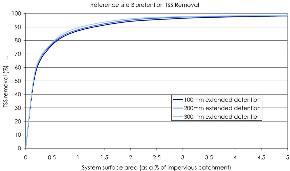
**Figure 4.4. TSS removal in bioretention systems with varying extended detention**
