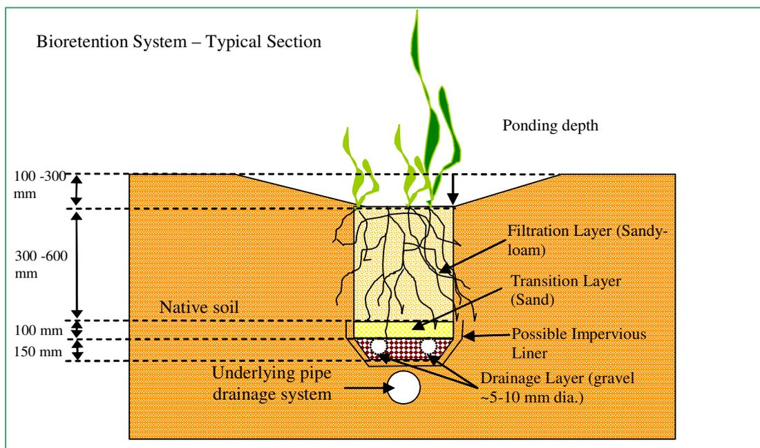
**Figure 5.2. Typical section of an bioretention basin**
