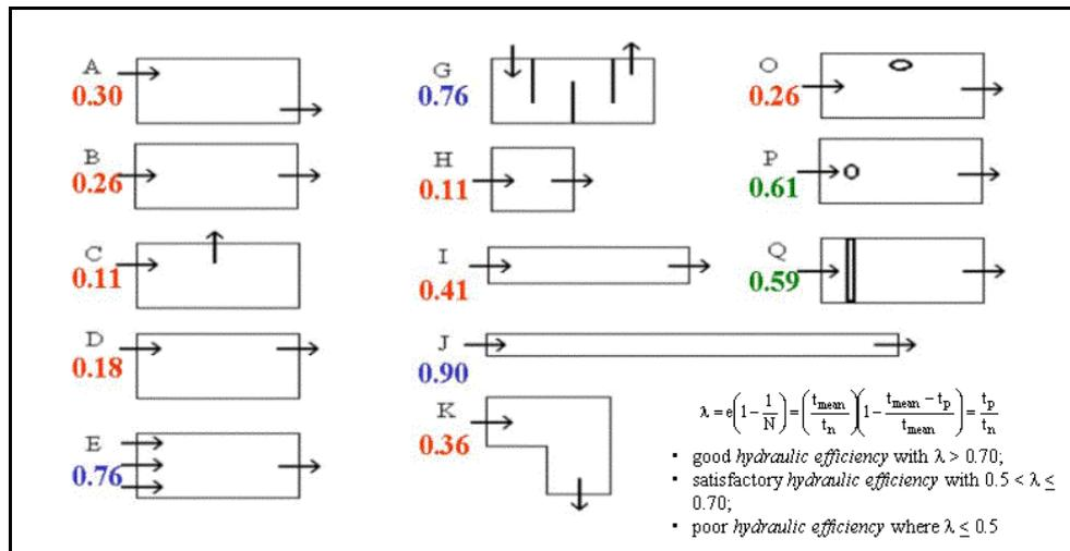
**Figure 8.6. Hydraulic Efficiency -  $\lambda$ - A measure of Flow Hydrodynamic Conditions in Constructed Wetlands and Ponds; Range is from 0 to 1, with 1 representing the best hydrodynamic conditions for stormwater treatment (Persson et al, 1999)**
