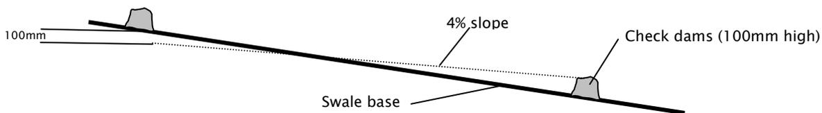
**Figure 7.14. Location of check dams in swales**
