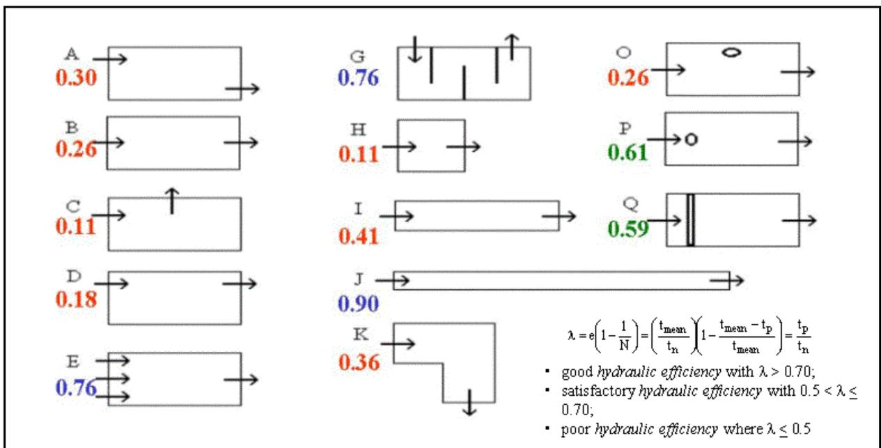
**Figure 3.3. Hydraulic Efficiency -  $\lambda$  - A measure of Flow Hydrodynamic Conditions in Constructed Wetlands and Ponds; Range is from 0 to 1, with 1 representing the best hydrodynamic conditions for stormwater treatment (Persson et al., 1999)**
