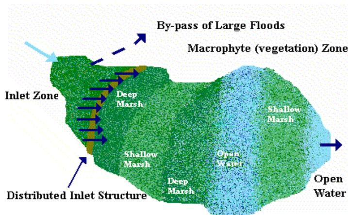
**Figure 8.5. Elements of a constructed wetland system**
