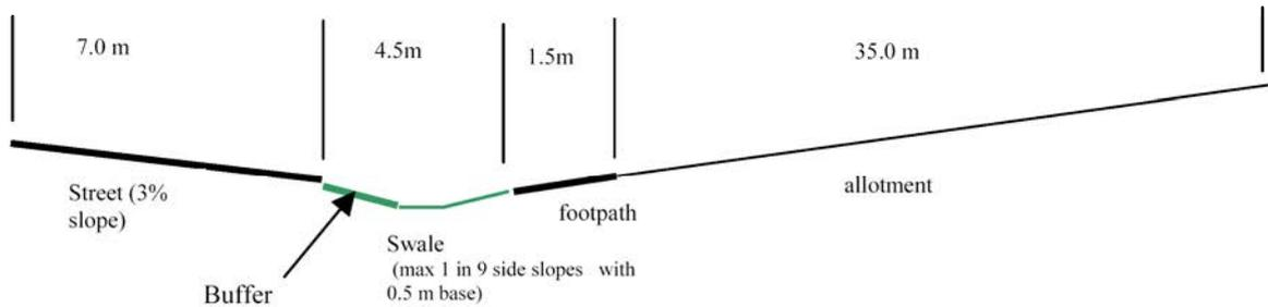
**Figure 7.15. Cross section of proposed buffer/swale system**
