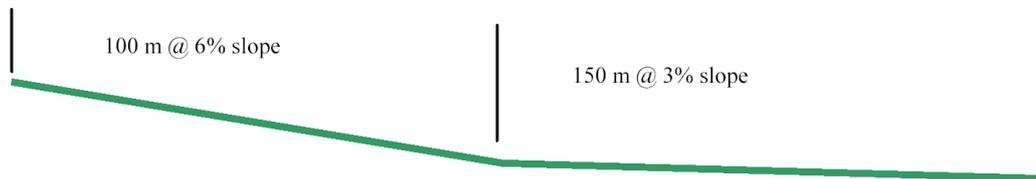
**Figure 7.16. Long section of proposed buffer/swale system**
