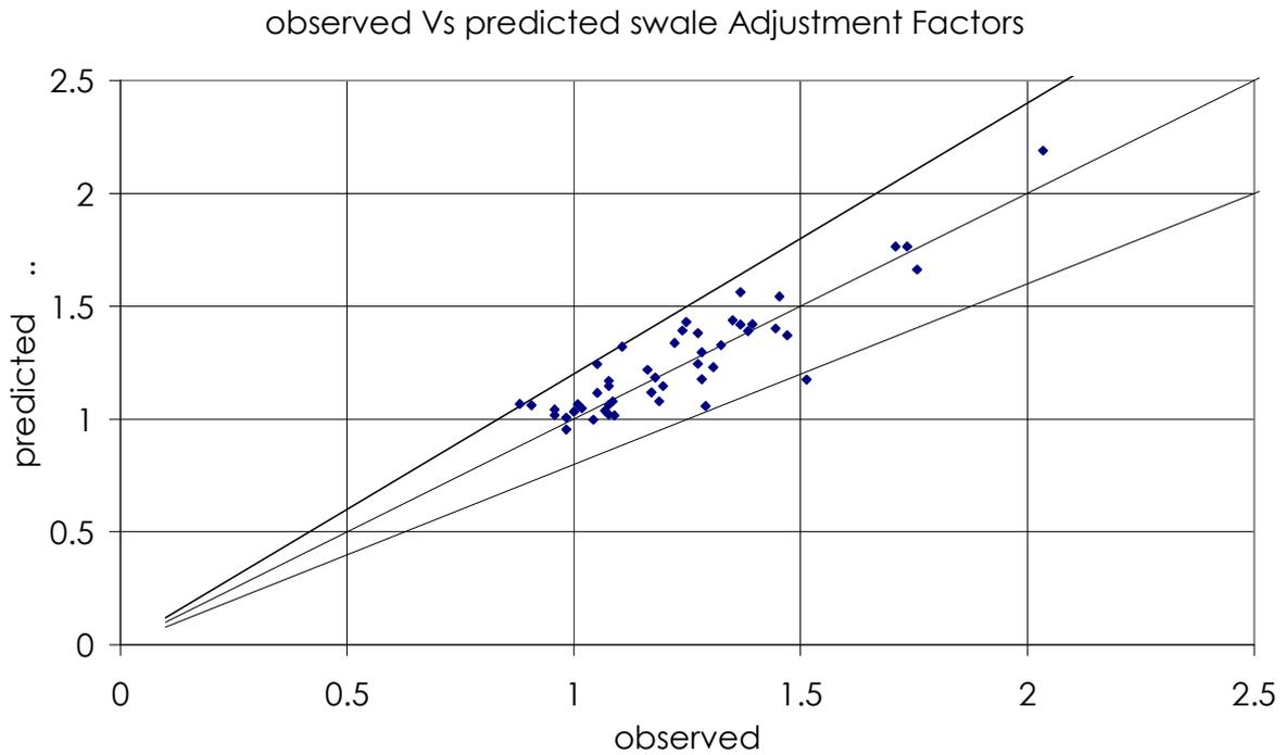
Figure A-10. Observed Vs predicted adjustment factors for grassed swales
