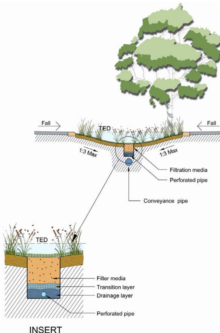
**Figure 4.1. Bioretention swale as a centre road median**
