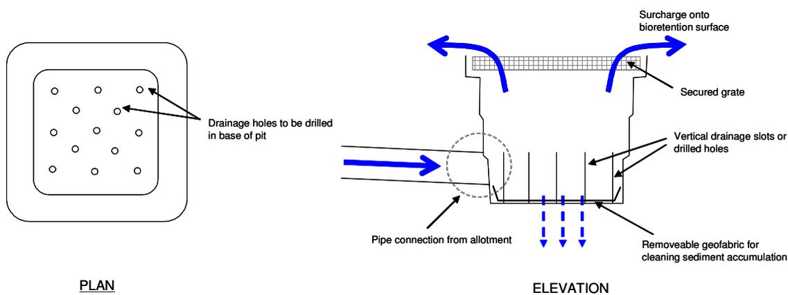
**Figure 4.10. Example of surcharge pit for discharging allotment runoff into a bioretention swale**
