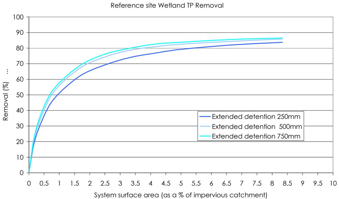
**Figure 8.3 TP removal in wetland systems with varying extended detention**
