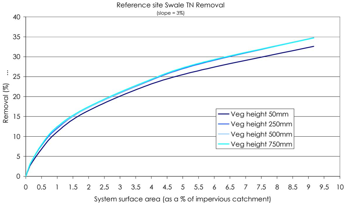
**Figure 7.9. TN removal in swale systems with varying vegetation height**
