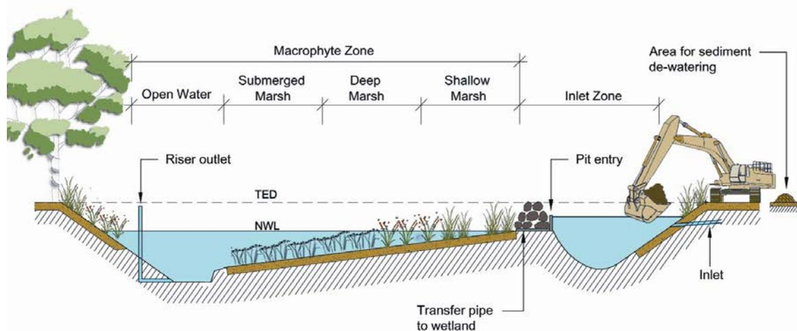
**Figure 8.1. Layout of a constructed wetland system**
