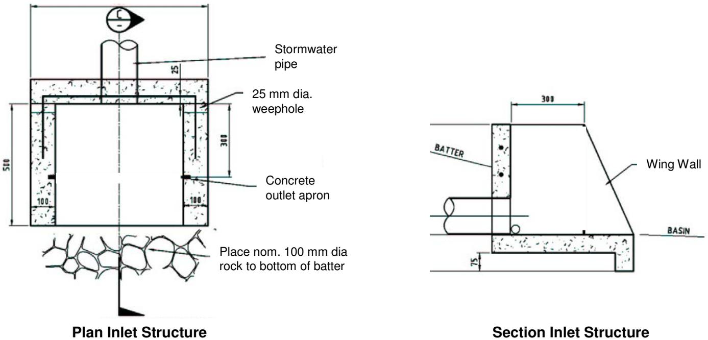
Provide energy dissipation and erosion protection in the form of rock beaching at the inlet structure;  $Q_{des} = 0.51 \text{ m}^3/\text{s}$ .
