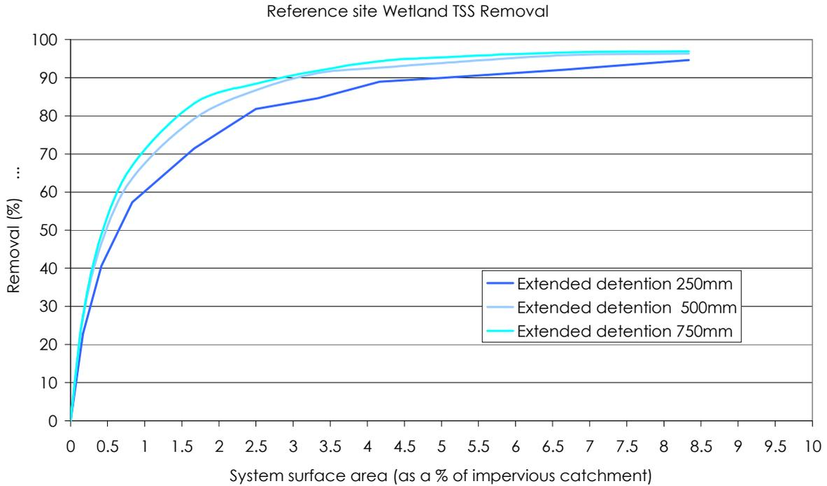
**Figure 8.2. TSS removal in wetland systems with varying extended detention**
