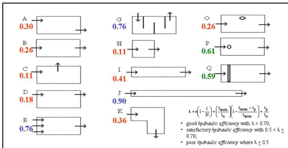
Figure 9.7. Hydraulic Efficiency -  $\lambda$  - A measure of Flow Hydrodynamic Conditions in Constructed Wetlands and Ponds; Range is from 0 to 1, with 1 representing the best hydrodynamic conditions for stormwater treatment (Persson et al., 1999)
