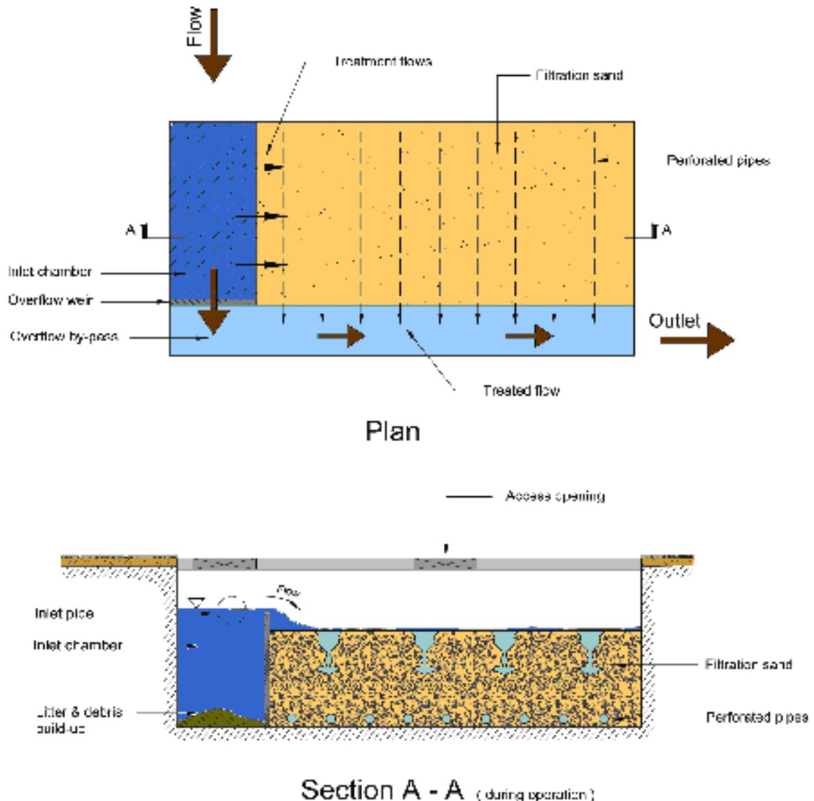
Figure 6.3. Illustration of a sand filter during operation
