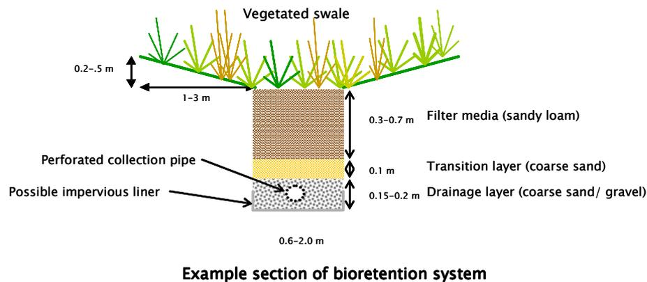
**Figure 4.3. Typical section of a bioretention swale**
