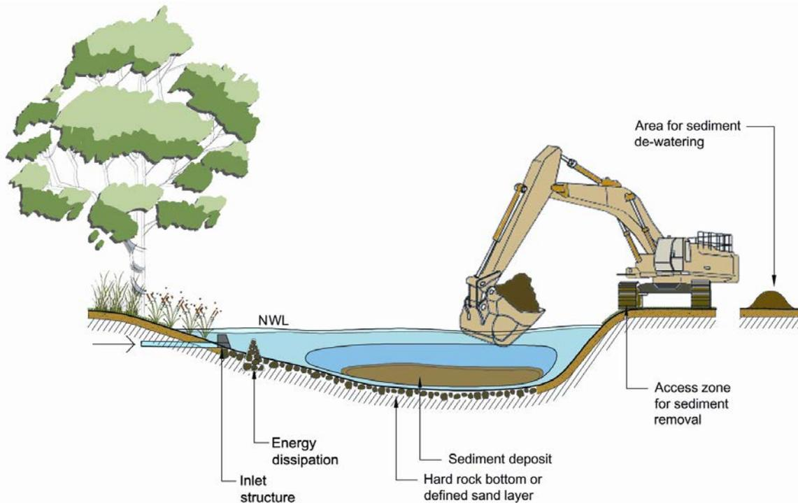
**Figure 3.1. Sedimentation basin layout**
