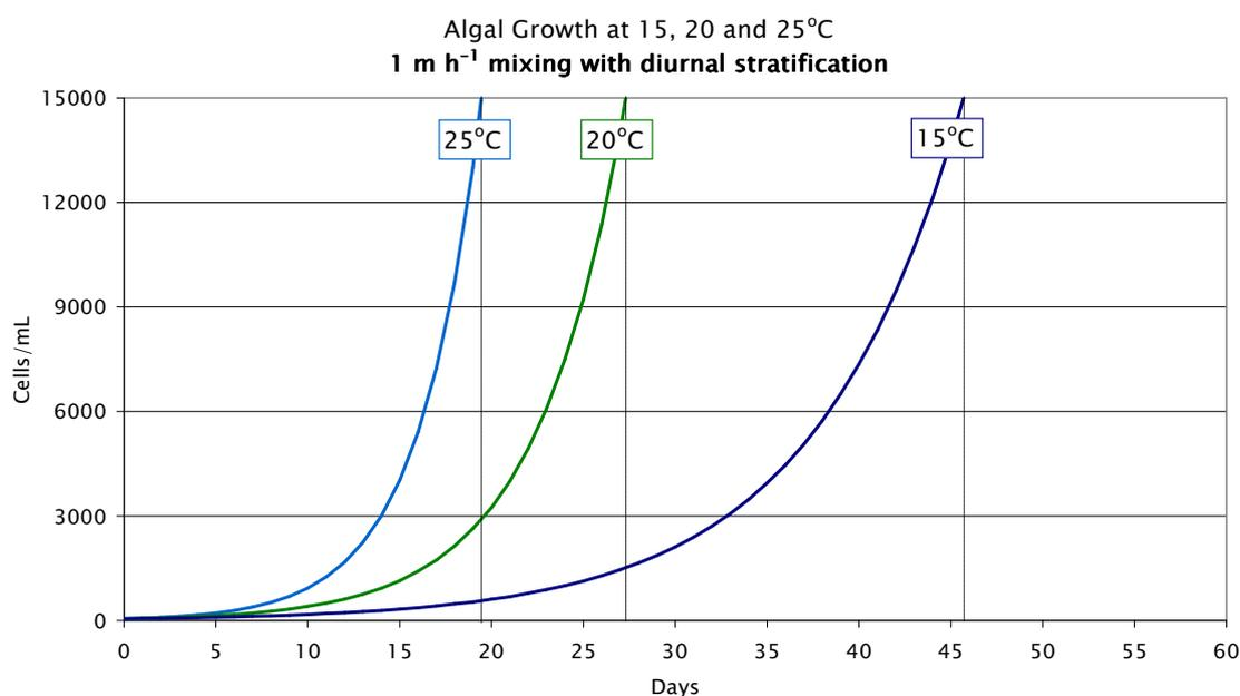
Figure D.4. Growth curves illustrating modelled times for cyanobacterial populations to reach bloom proportions under different temperature conditions and 1 m h<sup>-1</sup> mixing conditions with diurnal stratification. Based on growth rates of *A. circinalis* measured *in situ* (Westwood and Ganf, 2004) adjusted for temperature, Q<sub>10</sub> 2.9, and assuming 50 cells/mL starting concentrations.
