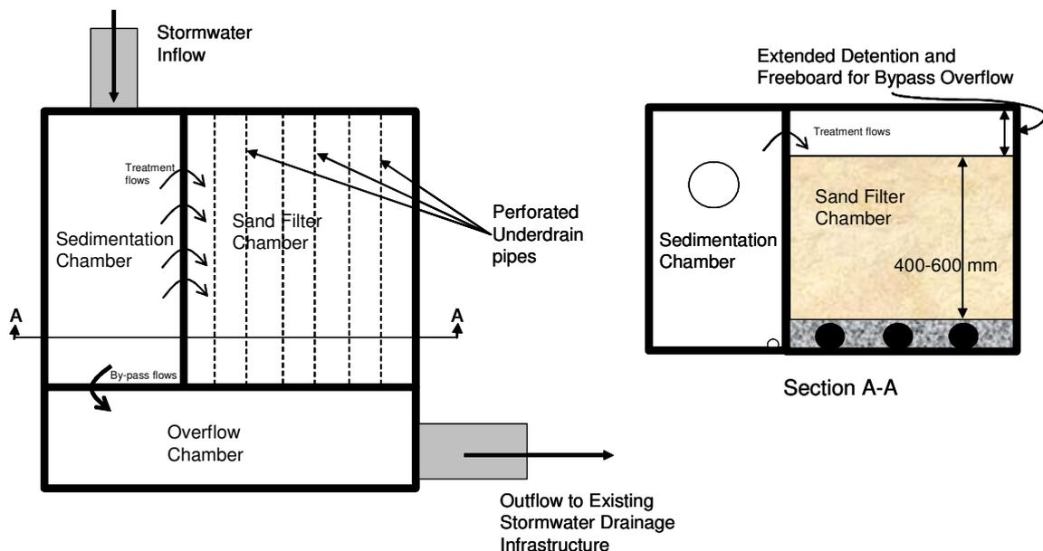
**Figure 6.1. Typical layout of a sand filter**
