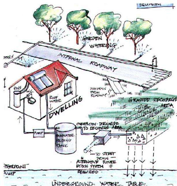
**Figure 10.4 Illustration of Allotment Stormwater Management Scheme**
