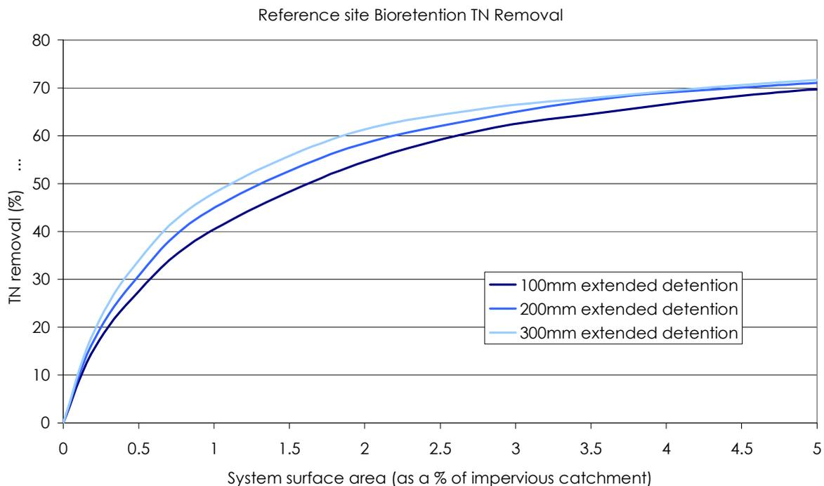
**Figure 5.5. TN removal in bioretention systems with varying extended detention**
