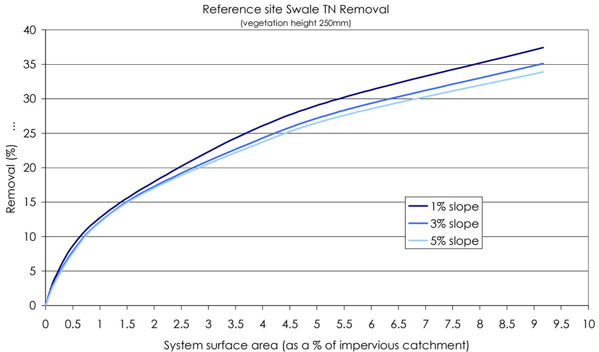
**Figure 7.6. TN removal in swale systems with varying slope**
