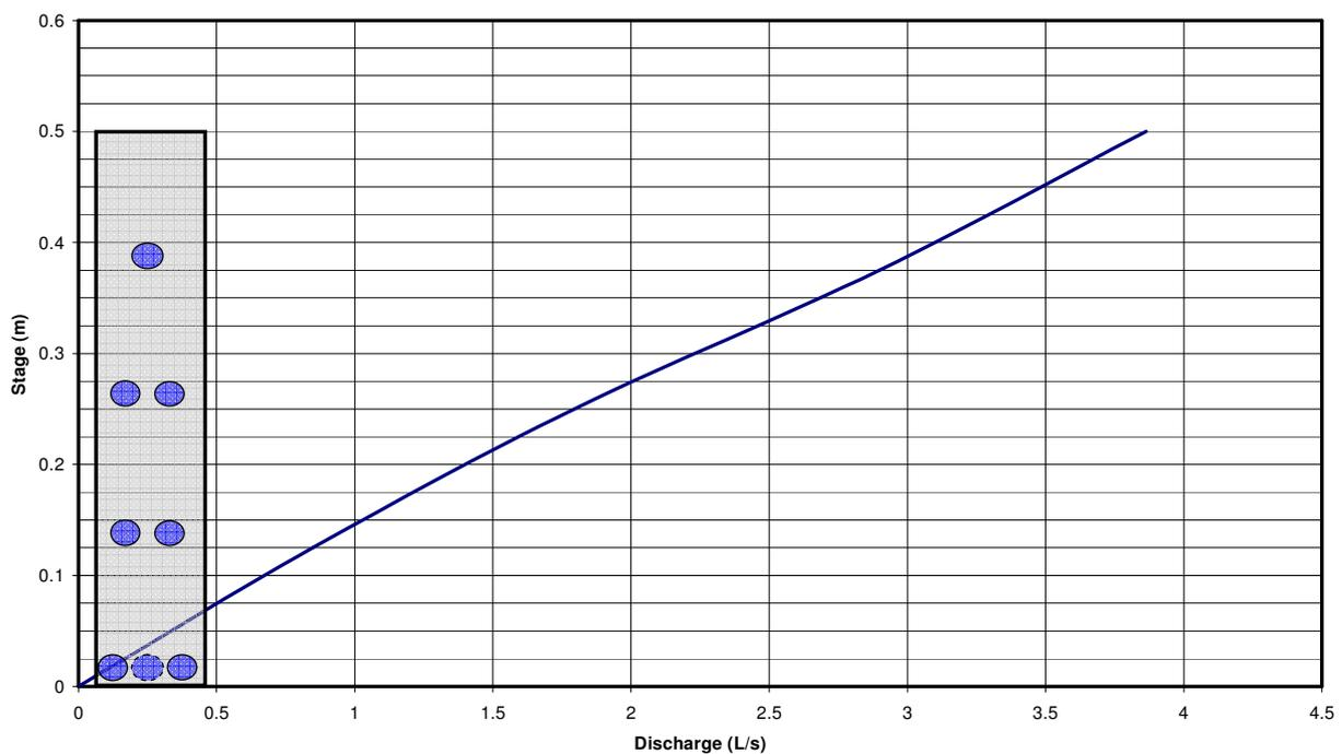
As the wetland is relatively small and the required orifices are small, it is necessary to include measures to prevent blocking of the orifices.
