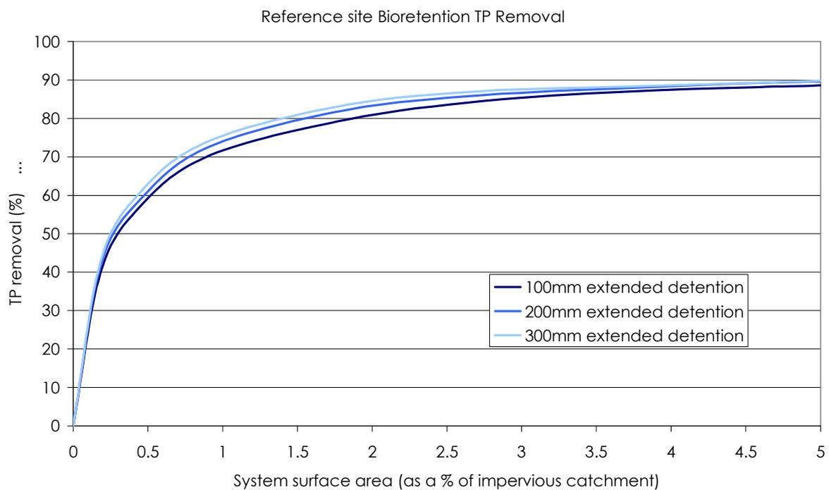
**Figure 4.5. TP removal in bioretention systems with varying extended detention**
