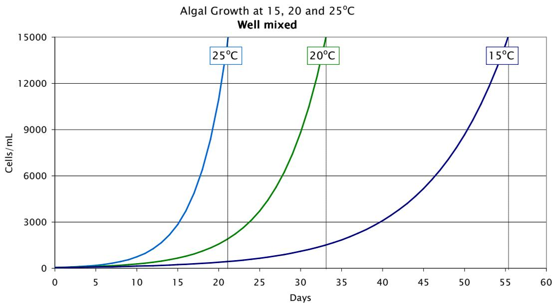
**Figure 9.5. Growth curves illustrating modelled times for cyanobacterial populations to reach bloom proportions under different temperature conditions and well mixed conditions. Based on growth rates of *A. circinalis* measured *in situ* (Westwood and Ganf, 2004) adjusted for temperature,  $Q_{10}$  2.9, and assuming 50 cells/mL starting concentrations.**
