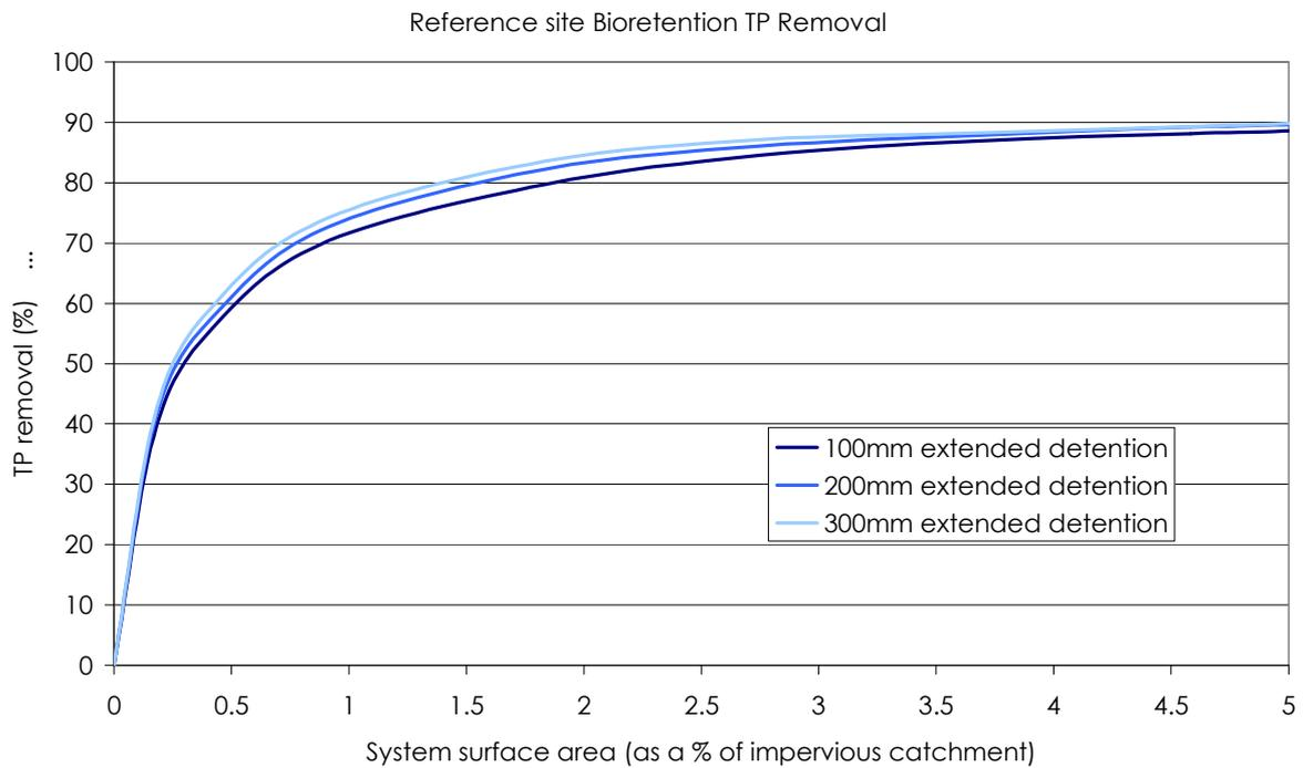
**Figure 5.4. TP removal in bioretention systems with varying extended detention**
