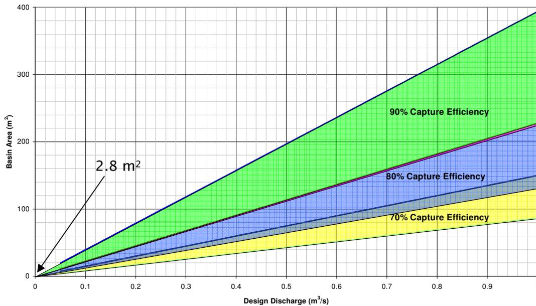
The available sediment storage is  $2.8 \times 0.6 = 1.68 \text{ m}^3$ . Cleanout is to be scheduled when the storage is half full. Using a sediment discharge rate of  $1.6 \text{ m}^3/\text{Ha}/\text{yr}$ , the clean out frequency is estimated to be:
