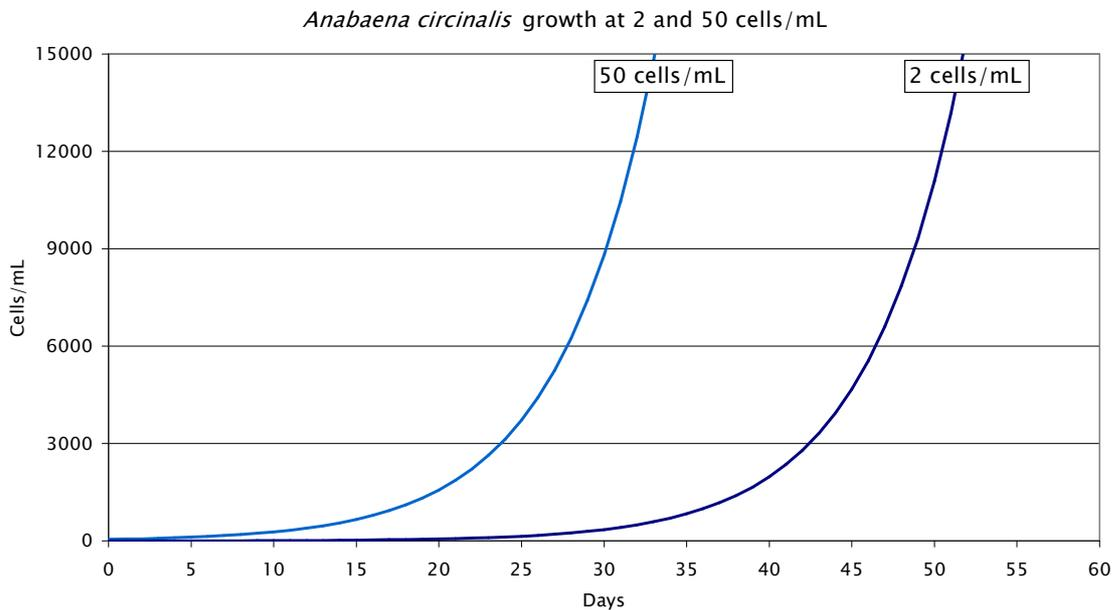
Figure D.3. Cyanobacterial growth curves at starting concentrations of 2 and 50 cells/mL. Constructed using growth rates of *A. circinalis* measured *in situ*, under well mixed conditions (Westwood and Ganf, 2004), adjusted for 20°C (Q<sub>10</sub> 2.9). The number of days taken to reach bloom proportions varies from 33 to 51 days depending on the starting cell concentration.
