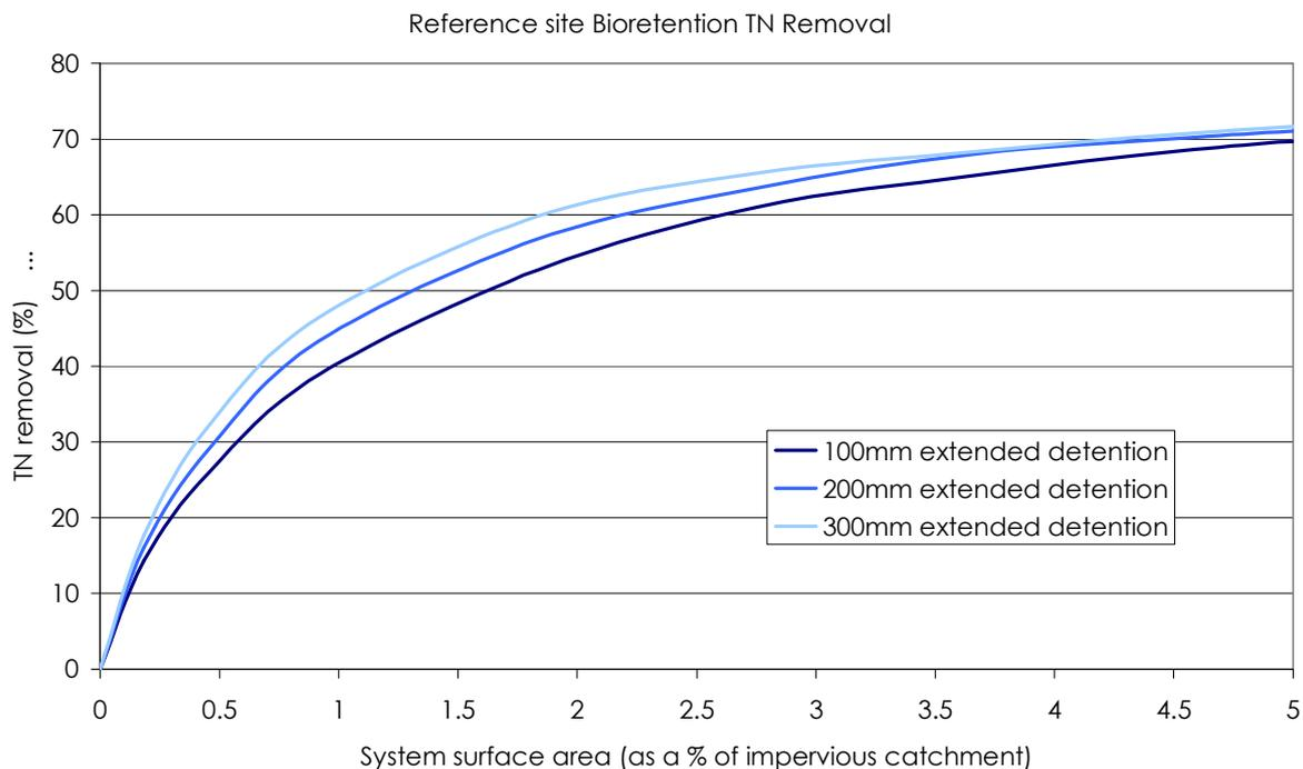
**Figure 4.6. TN removal in bioretention systems with varying extended detention**
