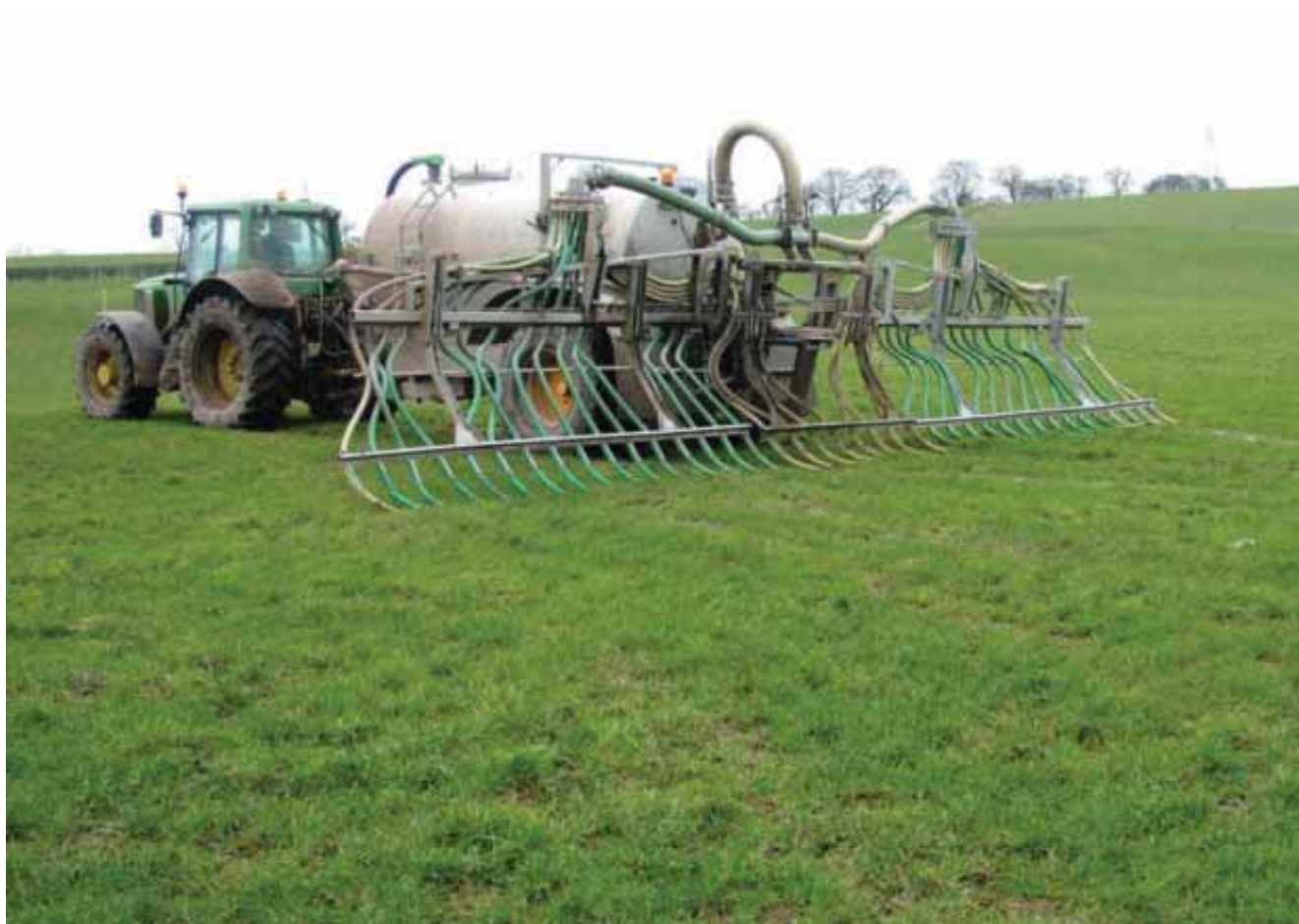
Injection of slurry to reduce ammonia emissions
