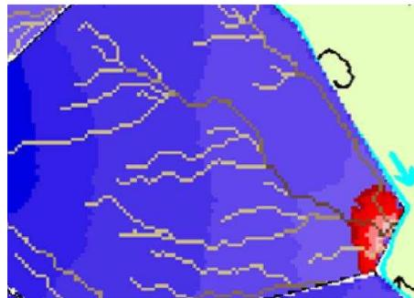
*Figure 16 – Lidar being used to identify overland flow pathways and low points*
