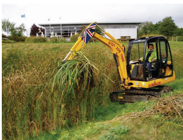
Managing wetland vegetation with a mini excavator. Larger excavators should not be necessary, motorway service area, M42
