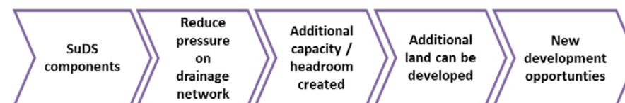
Figure 4-9 Impact pathway for enabling development
