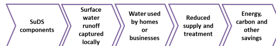
Figure 4-14 Impact pathway for rainwater harvesting
