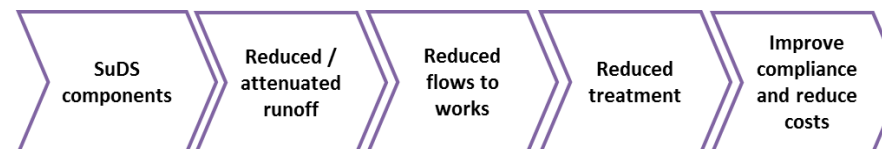
Figure 4-15 Impact pathway for sewage treatment
