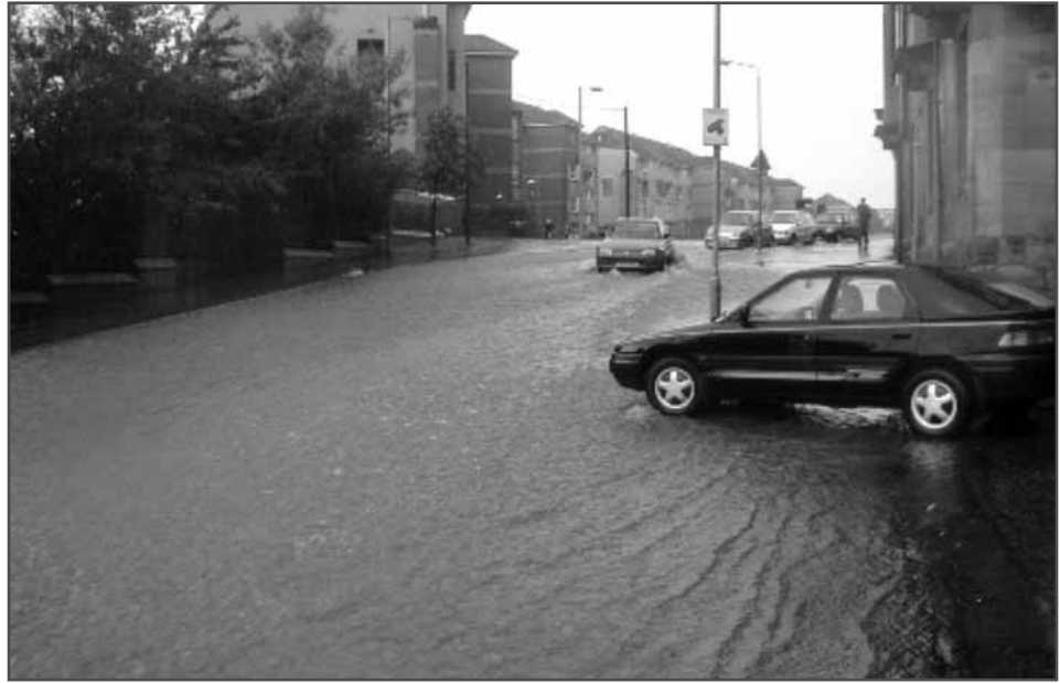
Figure 1.1 Highway acting as a flood pathway in an extreme rainfall event (courtesy Scottish Water)
