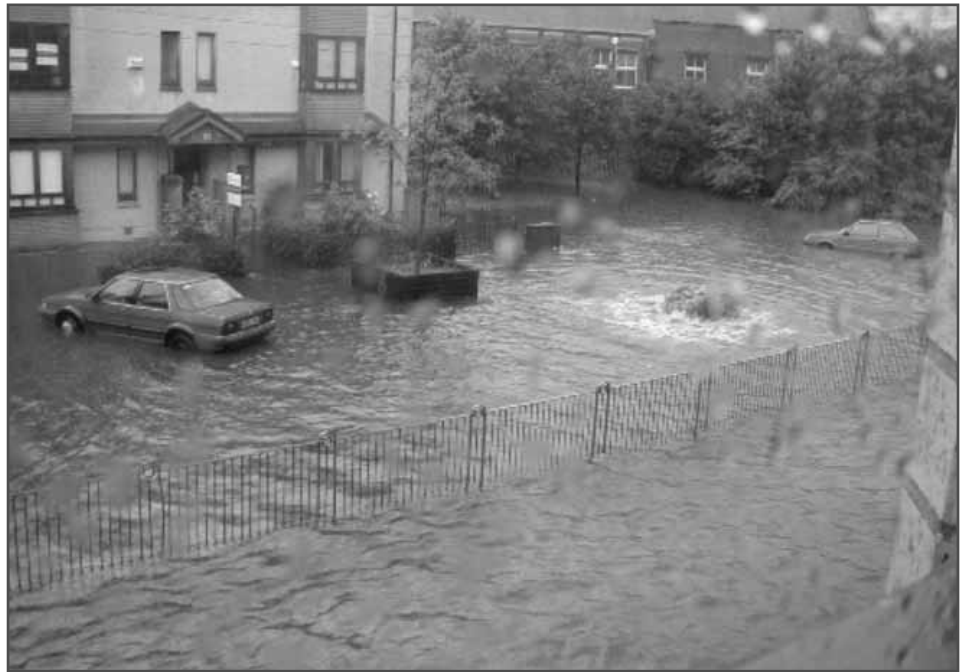
Figure 1.2 Property flooding from overloaded sewerage system (courtesy Scottish Water)
