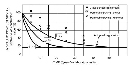
(b) : Hydraulic conductivity, k<sub>h</sub>, deterioration trend curve for porous and permeable paving filters subject to (fine) sediment loading, based on laboratory results (after Rommel et al, 2001; UWRC, 2002a and b)
