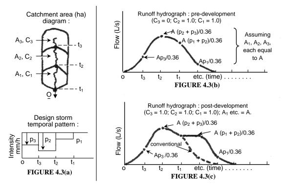
FIGURE 4.3 : Illustrations for hydrological analysis of 'top-end' sub-catchments
