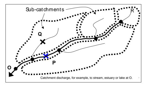
FIGURE 4.1 : Dendritic structure of a typical urban catchment
