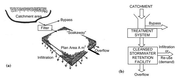
FIGURE 3.5 : Sketch of stormwater-retaining device and system schematic
