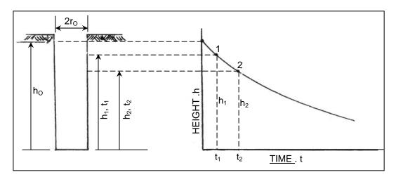
FIGURE 3.3 : Inverse augerhole test – definition of terms and typical "h" versus "t" relationship
