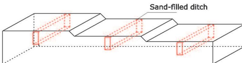
Fig. 2. Scheme of bench terraces with sand-filled ditches
