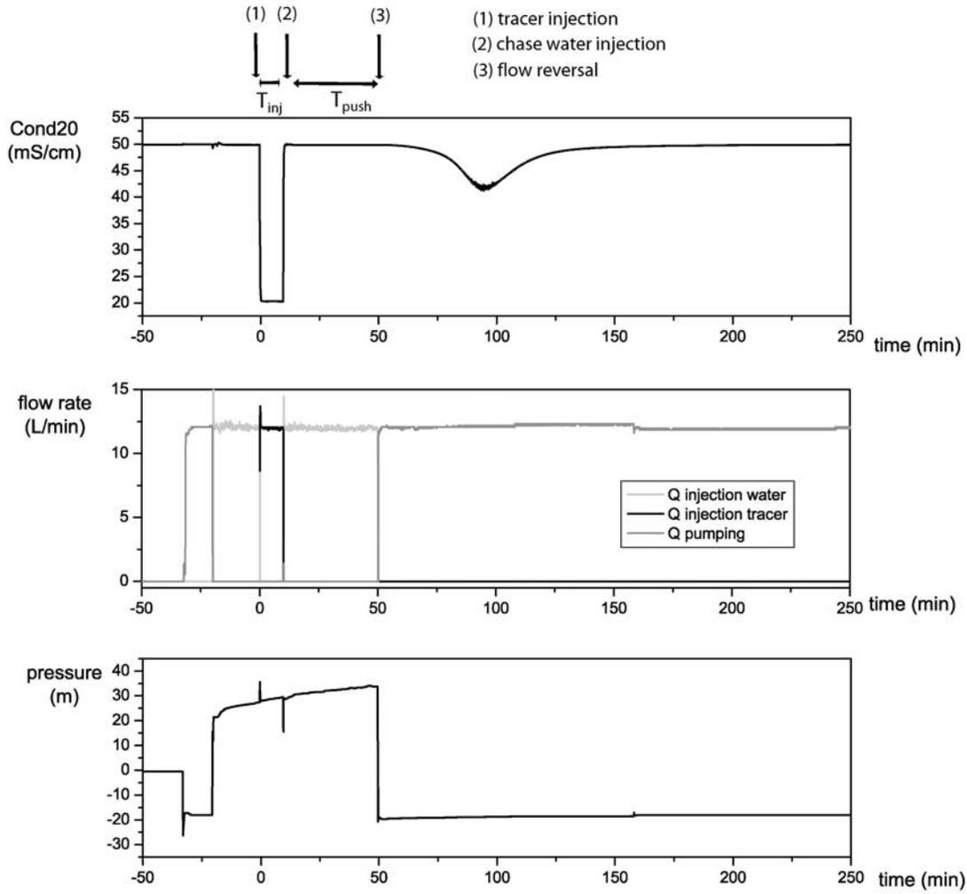
**Figure 7.** Example of SWIWT monitoring (tracer test 1–1). Evolution of (top) conductivity, (middle) flow rates, and (bottom) pressure as a function of time. The experiment was performed at 94 m depth. The tracer injection time is  $T_{inj} = 600$  s and the flushing water injection duration is  $T_{push} = 2400$  s. The flow rate is  $2 \times 10^{-4} \text{ m}^3 \text{ s}^{-1}$  (i.e.,  $12 \text{ L min}^{-1}$ ). The resident water conductivity is approximately 50 mS/cm.
