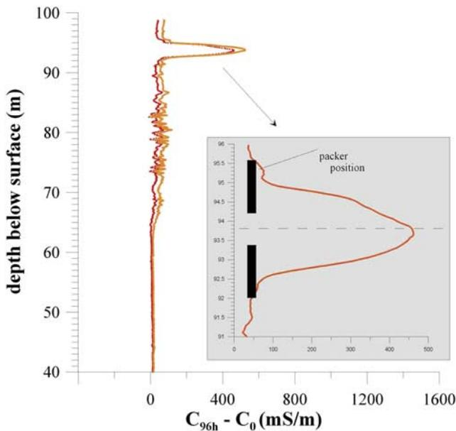
**Figure 9.** Difference between induction log in natural conditions ( $C_0$ ) and induction log 96 h after the injection of  $3 \text{ m}^3$  of freshwater between packers at 94 m in well MC2. The difference is shown as a function of depth for both the short- and long-range induction logs. The positive anomaly at 94 m marks out the location of the injected plume of freshwater 96 h after injection.
