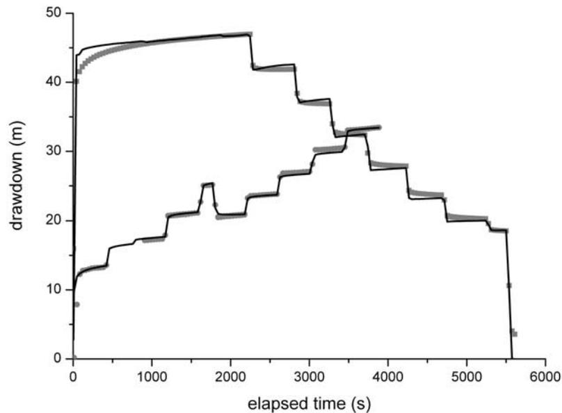
**Figure 5.** Step drawdown test results in the interval 93.55–94.35 m, with flow rates ranging between  $1.113 \text{ m}^3 \text{ s}^{-1}$  and  $3.073 \text{ m}^3 \text{ s}^{-1}$ . Dotted curves are measured data and continuous curves are outputs from the fitted model (transmissivity =  $1.6 \text{ m}^2 \text{ s}^{-1}$ ).
